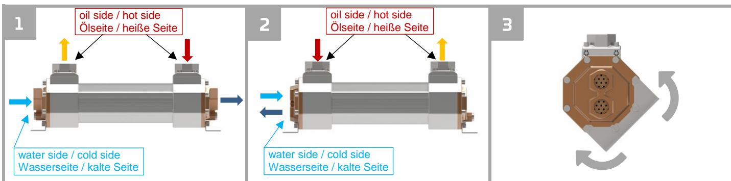
The heat exchanger should be mounted with the tube bundle axis in a horizontal position (parallel to the floor).
